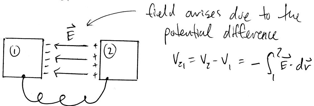
\* p-type and n-type semiconductor brought into contact
