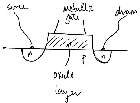
→ variable mode of operation depending on whether a voltage is applied to the gate
