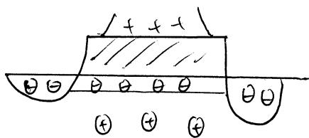
an "inversion layer" with majority electron carriers is established that connects source to drain
