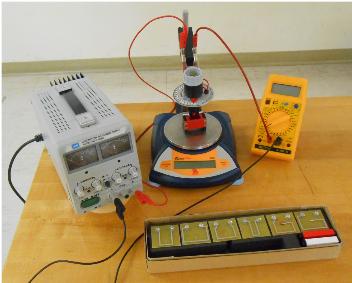
Figure 18.1: Current Balance Arrangement for Varying Current or Length
