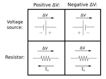
1. Use Kirchhoff's Voltage Law to find the missing voltage differences in the following circuits. For these circuits, current flows clockwise and potential difference is measured clockwise. (4 pts)
