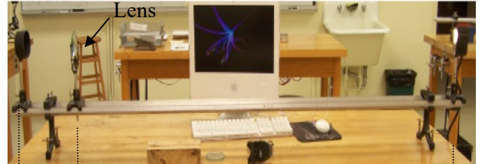
Figure 27-1 Conjugate Foci Method - 1 st measurement
