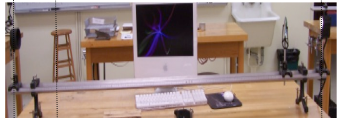
Figure 27-2 Conjugate Foci Method - 2 nd measurement
