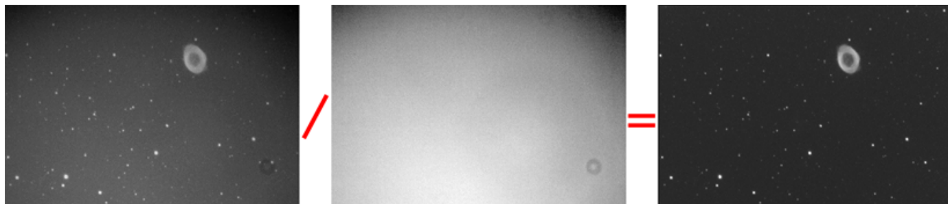
Fig. 9: Dividing by a flat frame removes uneven shadows. In the raw image, far left, notice the darker background top right, as well as the blob bottom right of the image. Flat fielding divides off both.
