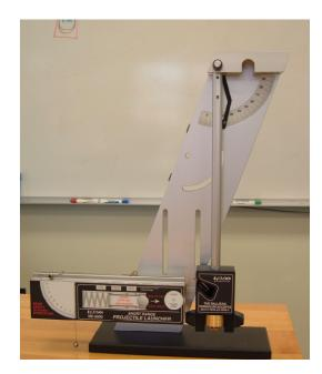
Fig. 8-1 Ballistic Pendulum
