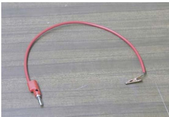
**Fig.8-3** Banana-Alligator Wire Lead
