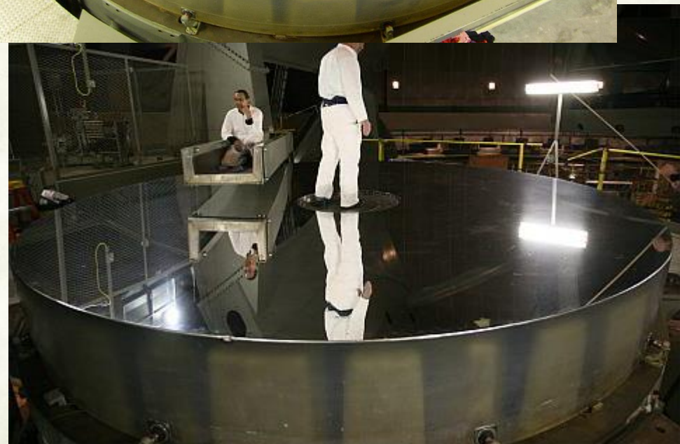
5m mirror of the Mt. Palomar telescope, aluminum layer stripped. Cleaning for recoating (weight 14.5 tons; thick to make them rigid and won't deform under own weight )
