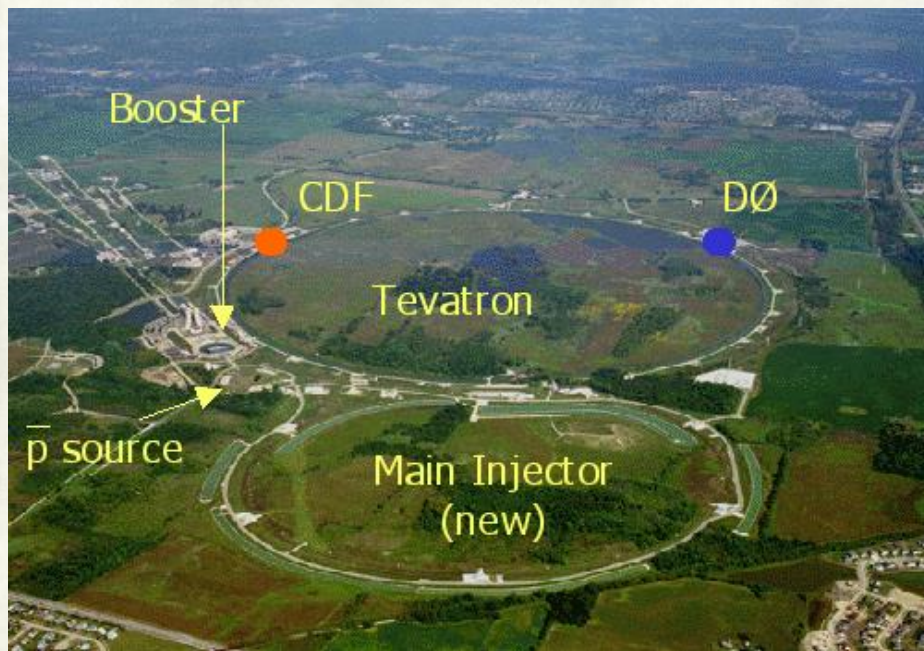
Accelerator complex at the Fermilab, near Chicago (accelerator ring diameter: 2 km)
