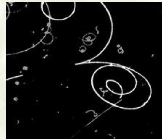
Tracks of an electron-positron pair produced from a \gamma ray inside a particle detector
