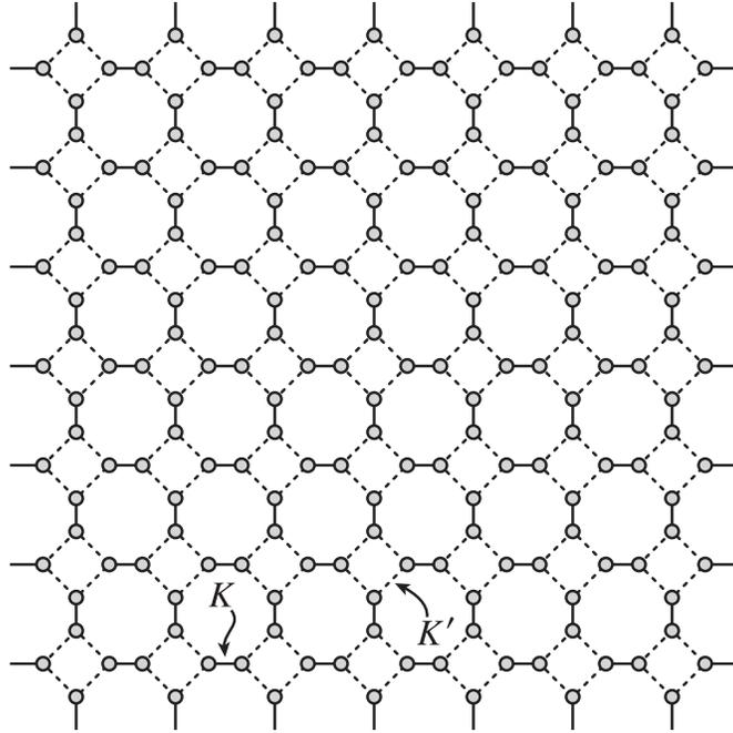
16. Here's the same lattice from the previous question, where the lines now represent two types of covalent bond. The solid lines denote bonds of equilibrium length  $a$  and Hooke's law spring constant  $K$ ; the dashed lines denote bonds of length  $\sqrt{2}a$  and spring constant  $K'$ .
