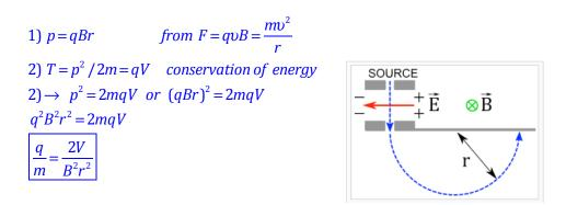
2- Derive the Mass Spectrometer Equation.  $m = q \frac{B^2 x^2}{8V}$  where B is the magnetic field intensity, x is the distance to each peak, and V is the ion accelerating voltage.
