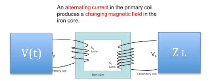
Assume  $V_p(t) = V_1 e^{i\omega t}$  and a load  $Z_L$  is attached to the secondary. Let I1 and I2 be clockwise currents in the primary and secondar coils. We can write Kirchoff's:
