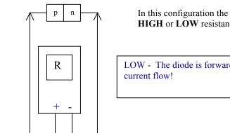
In this configuration the resistance meter reads a **HIGH** or **LOW** resistance for the diode? Explain.
