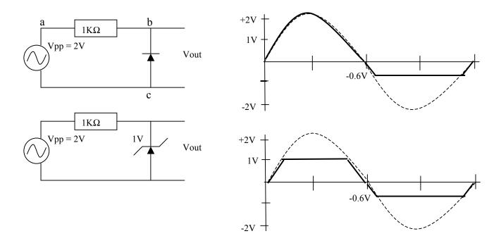
**Case-1:** The diode is reversed biased on the  $1^{st}$  half-cycle.and has infinite resistance. All voltage is dropped across it, implying no current flow, Vac=Vb. On the negative voltage down cycle the same occurs until the voltage Vbc~ -0.6V and the resistance across the diode drops to zero. Vbc remains at -0.6V
