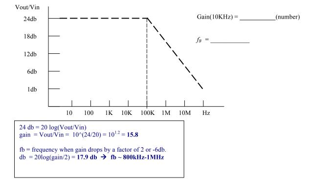
**#8-** The gain versus frequency of an amplifier is shown below. What is the gain of this amplifier at f = 10KHz? What is the break frequency  $f_B$  of the amplifier ?
