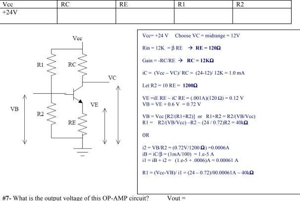
**#6-** Design a common emitter transistor amplifier with gain of -100 and input impedance of  $12K\Omega$  using an npn transistor  $\beta$ = 100. Place your resistor parameters in the boxes.
