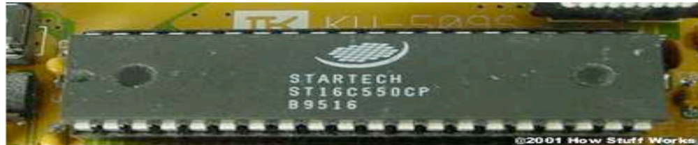
This 40-pin Dual Inline Package (DIP) chip is a variation of the National Semiconductor NS16550D UART chip.
