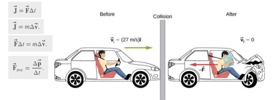
The motion of a car and its driver at the instant before and the instant after colliding with the wall. The restrained driver experiences a large backward force from the seatbelt and airbag, which causes his velocity to decrease to zero. (The forward force from the seatback is much smaller than the backward force, so we neglect it in the solution.)
