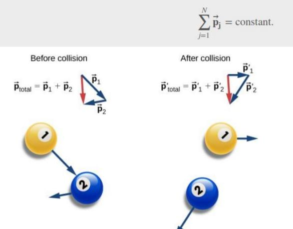
Before the collision, the two billiard balls travel with momenta  $\vec{p}_1$  and  $\vec{p}_3$ . The total momentum of the system is the sum of these, as shown by the red vector labeled  $\vec{p}_{total}$  on the left. After the collision, the two billiard balls travel with different momenta  $\vec{p}'_1$  and  $\vec{p}'_3$ . The total momentum, however, has not changed, as shown by the red vector arrow  $\vec{p}'_{total}$  on the right.
