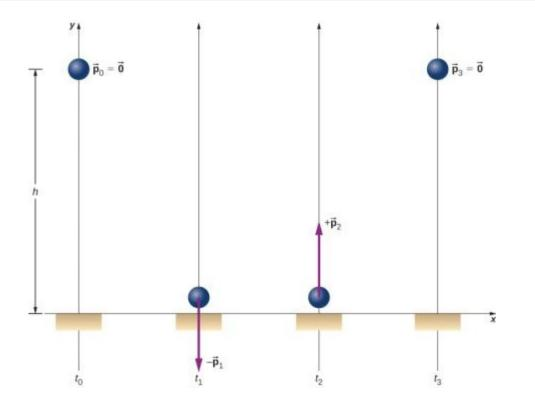
A superball is dropped to the floor ( $t_0$ ), hits the floor ( $t_1$ ), bounces ( $t_2$ ), and returns to its initial height ( $t_3$ ).
