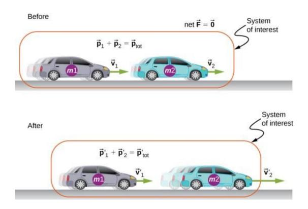
The two cars together form the system that is to be analyzed. It is important to remember that the contents (the mass) of the system do not change before, during, or after the objects in the system interact.
