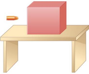
After striking the block, the bullet is embedded in the block and the block and the bullet move together as one unit.
