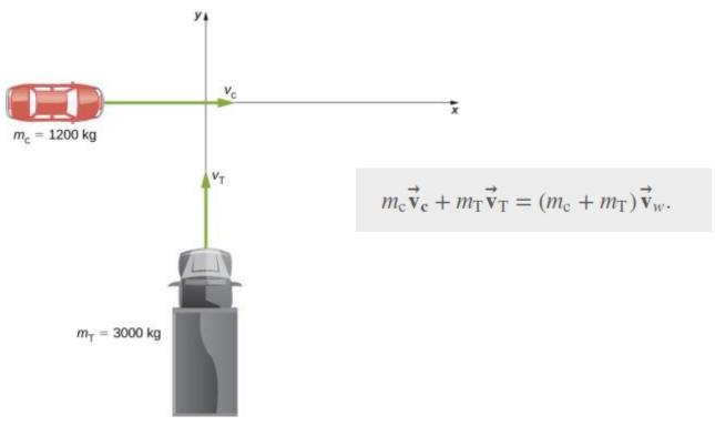
A large truck moving north is about to collide with a small car moving east. The final momentum vector has both x- and y-components.
