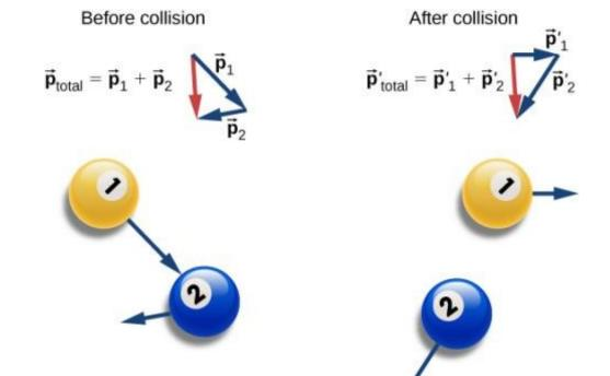
Before the collision, the two billiard balls travel with momenta  $\vec{p}_1$  and  $\vec{p}_3$ . The total momentum of the system is the sum of these, as shown by the red vector labeled  $\vec{p}_{total}$  on the left. After the collision, the two billiard balls travel with different momenta  $\vec{p}'_1$  and  $\vec{p}'_3$ . The total momentum, however, has not changed, as shown by the red vector arrow  $\vec{p}'_{total}$  on the right.
