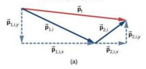
Add x and y components to obtain x and y components of final momentum
