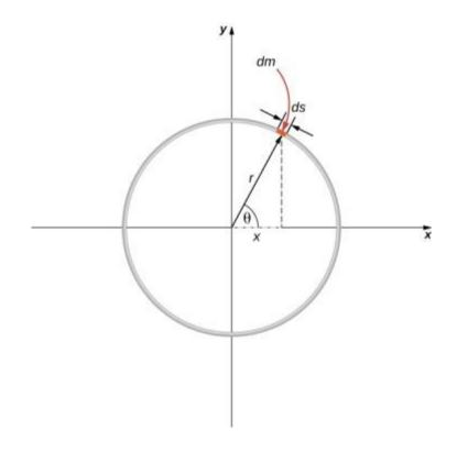
Finding the center of mass of a uniform hoop. We express the coordinates of a differential piece of the hoop, and then integrate around the hoop.
