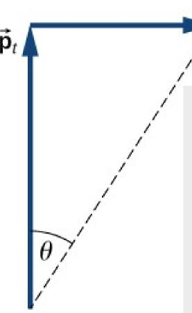
Graphical addition of momentum vectors. Notice that, although the car's velocity is larger than the truck's, its momentum is smaller.
