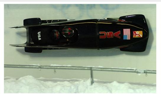
From racing cars to bobsled racers, aerodynamic shaping is crucial to achieving top speeds. Bobsleds are designed for speed and are shaped like a bullet with tapered fins. (credit: "U.S. Army"/Wikimedia Commons)
