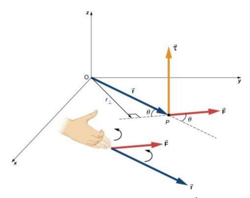
The torque is perpendicular to the plane defined by  $\vec{r}$  and  $\vec{F}$  and its direction is determined by the right-hand rule.
