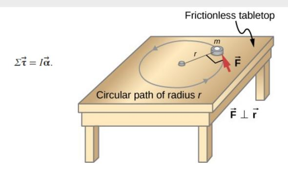
An object is supported by a horizontal frictionless table and is attached to a pivot point by a cord that supplies centripetal force. A force  $\vec{\mathbf{F}}$  is applied to the object perpendicular to the radius r, causing it to accelerate about the pivot point. The force is perpendicular to r.
