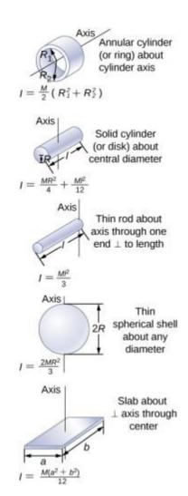
Values of rotational inertia for common shapes of objects.
