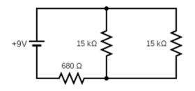
13) Looking at the schematic, visualize the electric current as something analogous to water that is flowing through the circuit. Using this model, can you make quantitative sense of the current measurements that you took? How do the three current measurements relate to each other?
