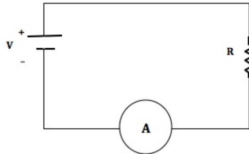
2. Consider the behavior of the above circuit when altered in the following manner. Voltage and resistance are both increased; the current in the circuit will be: (3 pts)
