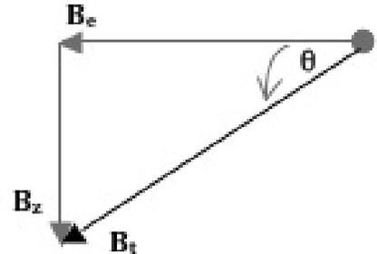
10. Compare your measured  $B_t$  from this experiment to a sample value of  $43 \mu\text{T}$ , the magnitude of the magnetic field in Tucson, Arizona. (6 pts)
