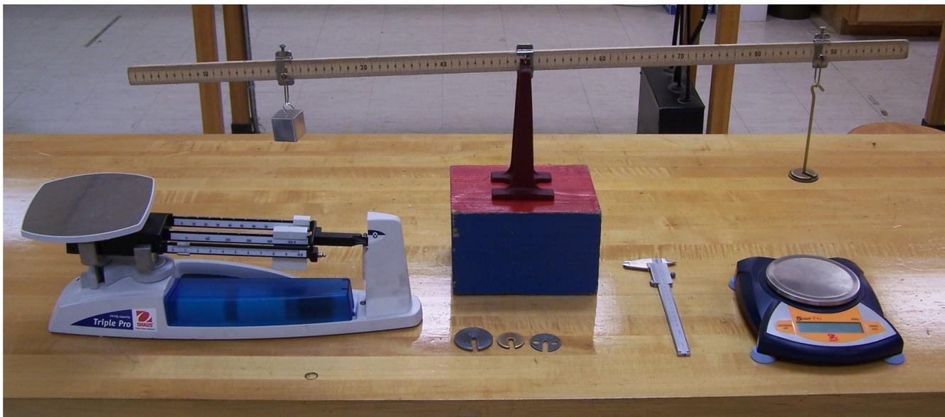
Figure 8.1: The wood block provides necessary height for the hangers to not touch the table.
