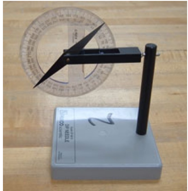
Figure 18.6: Dip Needle: Vertical Orientation
