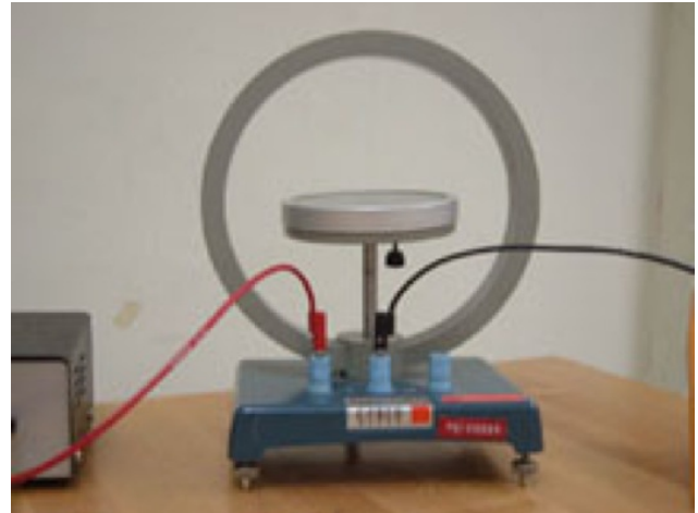
Figure 18.9: Side View - Compass located inside wire loops.
