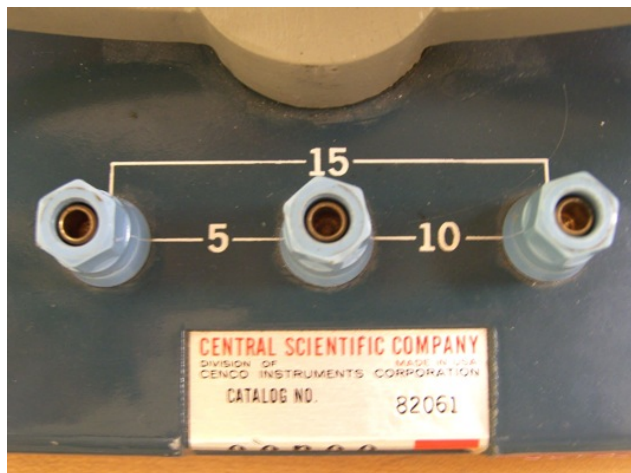
Figure 18.12: If leads are plugged into the left and middle jacks, N = 5 , as indicated. If plugged into the right and middle jacks, N = 10 . If plugged into the left and right jacks, N = 15 .
