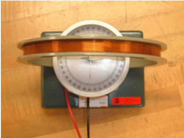
Figure 18.8: Top View - Wire loops encircle compass.
