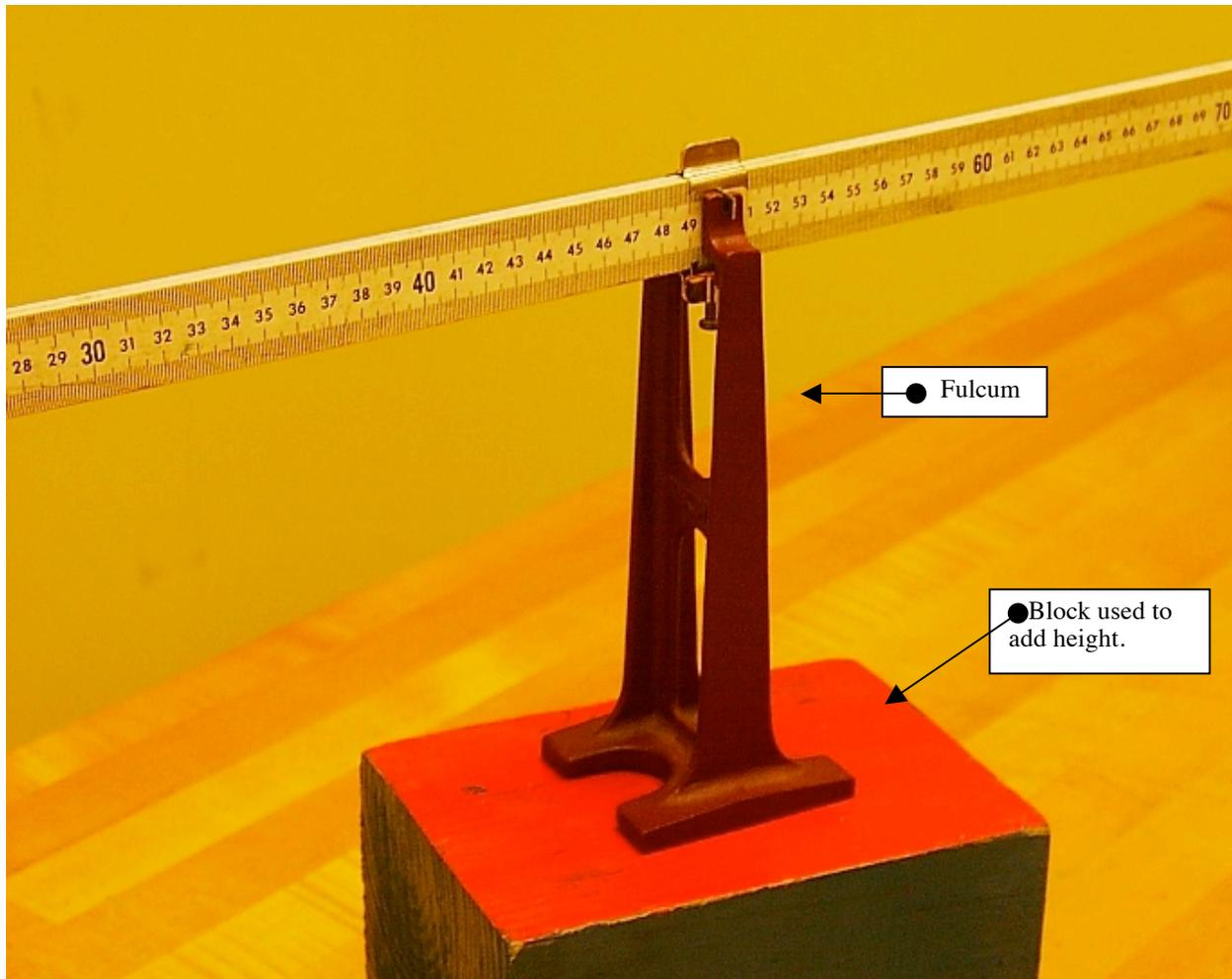
Fig. 9-1 Torque Apparatus
