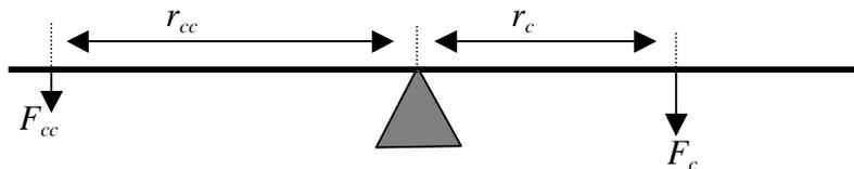
Fig 9-2 Torque components,  $F$  (force) and  $r$  (moment arm).
