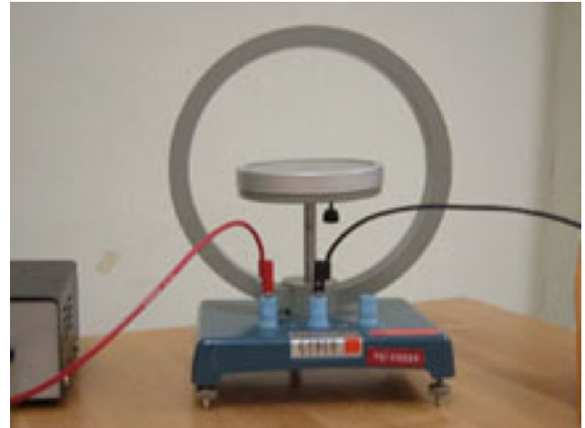
Figure 17.9: Side View - Compass located inside wire loops.
