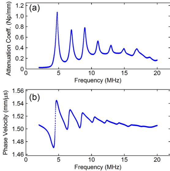
FIG. 2 (color online). (a) The attenuation coefficient and (b) the phase velocity spectra for the microsphere suspension.
