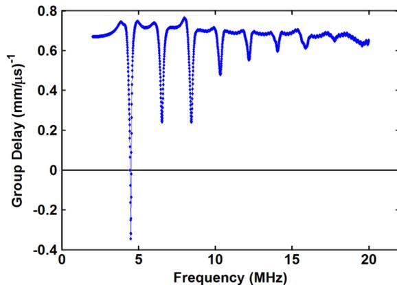
FIG. 3 (color online). The group delay spectrum for the microsphere suspension. The negative delay band runs from 4.45 to 4.53 MHz.
