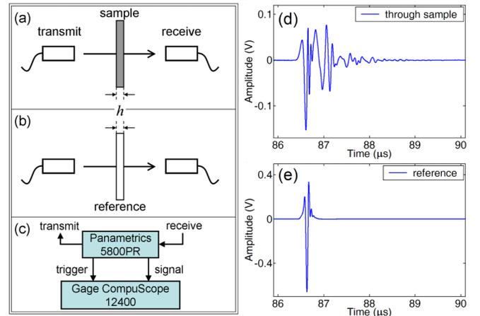
FIG. 1 (color online). (a) The through-sample and (b) reference signal acquisition steps of the substitution method. (c) Diagram of the measurement system. (d) The through-sample and (e) reference waveforms (4096 averages).
