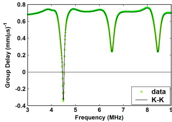
FIG. 5 (color online). A comparison of the measured group delay with the predicted spectrum from Kramers-Kronig relations. The plot is zoomed to resolve the negative delay band.
