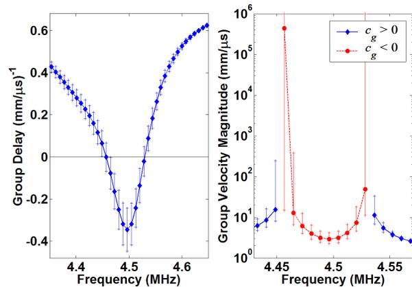
FIG. 4 (color online). (a) The group delay spectrum, zoomed in to resolve the negative delay band. (b) The group velocity magnitude in the abnormal region plotted logarithmically. This is the absolute value of the inverse of the delay curve. The maximum velocity magnitude is  $4.34 \times 10^5$  mm/ $\mu$ s at 4.46 MHz.
