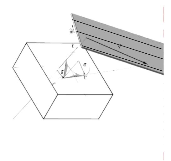
$\alpha$  is perpendicular to t and has magnitude  $\alpha$ . For small enough  $\alpha$  This vector is  $\hat{t}' - \hat{t}$ . The vector  $\delta$  is perpendicular to t and has the magnitude delta. And V is the vector connecting the points where the undeviated track would intersect the plane to the place where the multiple scattered track actually intersects it.
