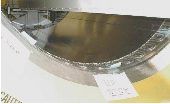
Fig. 6. Barrel panels in place at the inside of the electromagnetic calorimeter.
