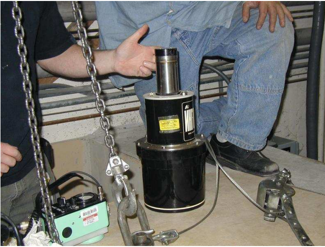
Fig. 3. The neutron-generating unit of the neutron generator system.
