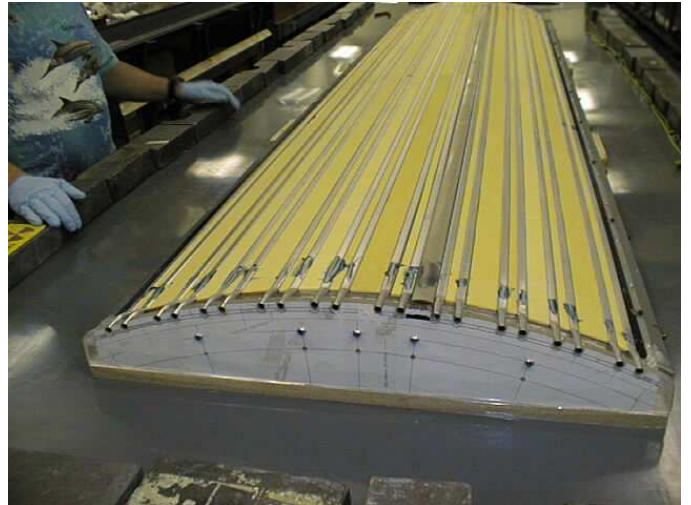
Fig. 5. Fabrication of the barrel panels with the top aluminum shield still missing. One can see the flattened aluminum tubes running up and down embedded in polyurethane.
