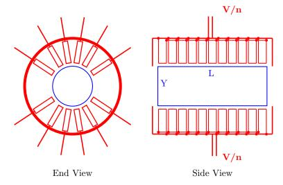
For this case, we can write the 2D fields in the long magnet limit. Let the inner and outer radii of the coils be  $r_1$  and  $r_2$ , and I be the total current in all loops on one side. Then if  $i_1$  is the current density on the inside of the loops,  $i_2$  is the current density on the outside of the loops, and  $i_3$  is the current density on the shield can. Defining
