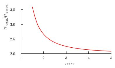
It is seen that, for a ratio of  $r_2/r_1 = 3$  the stored energy is increased by a factor of 2.25. Including the factor for the cylindrical case and dividing by the previously assumed value of  $f_{\Phi}$ , we obtain an estimated energy and current factor of 1.7 times that of the rectangular ferrite example. Despite the higher currents and stored energy, this solution has the advantages that
