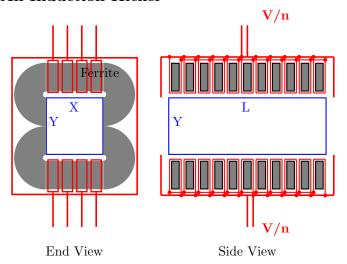
In this concept, the pulsed conductors are wound around the flux return yokes, instead of around the beam aperture its self. The windings can now be broken into many (n) separate loops, each about a sub section of the yoke. The windings are connected in parallel, so the current increases, but the voltage is reduced by the factor 1/n, and can be chosen to match a magnetic amplifier driver (typical Voltage 190 kV, requiring  $n \approx 30$ : 15 on each side, each 7 cm thick).
