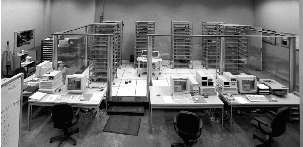
Figure 5.1: Mississippi farm overview. Servers are on the four tables. Clients are on the racks shown and on desktops not shown. One third of E791's 50 Terabyte raw data set was reconstructed in Mississippi.
