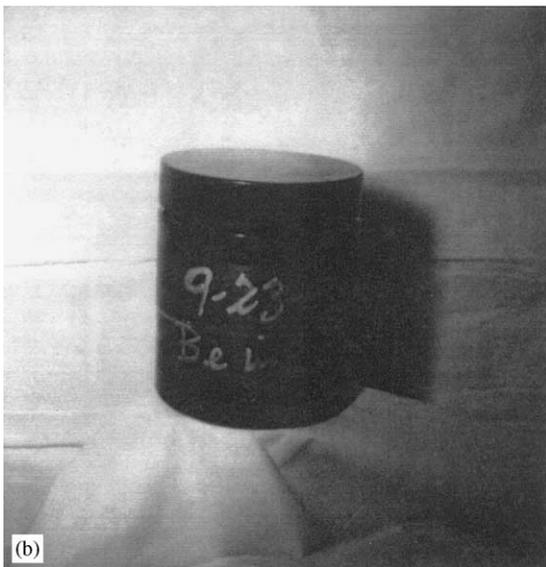
Fig. 3. Photos of the glass jar: (a) before and (b) after irradiation. It shows how dark in color the glass jar became after the irradiation.
