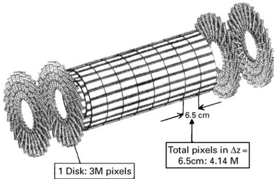
Fig. 1. A perspective figure of the pixel tracker of the CMS. It shows two layers of barrel pixels and two forward discs. We plan to have three barrel layers and three forward discs in the final configuration.
