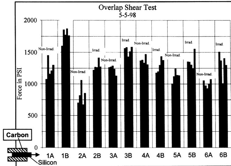
Fig. 5. A histogram plot of the results. It shows that there are small variations in five samples for each epoxy: (1A and 1B) Epon 815–80 EM-308; (2A and 2B) Epon 815–13 TETA; (3A and 3B) Epon 815–50 Epon V-40; (4A and 4B) Epon 815–70 Epon V-50; (5A and 5B) (80 D.E.R. 332+20 D.E.R. 732)-13 TETA; (6A and 6B) (80 D.E.R. 332+20 D.E.R. 736)-13 TETA. Each Sample A has not been irradiated, but each Sample B has been irradiated.
