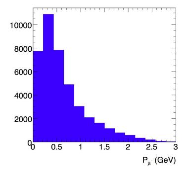
Figure 1: Belle II simulated muon momentum from  $\bar{B}_d^0 \to D^{*+} \mu^- \bar{\nu}_{\mu}$  decays. Note that many of the muons are too low in momentum to be identified by the KLM range detector. However, the ITOP Cherenkov may be able to identify low momentum muons.
