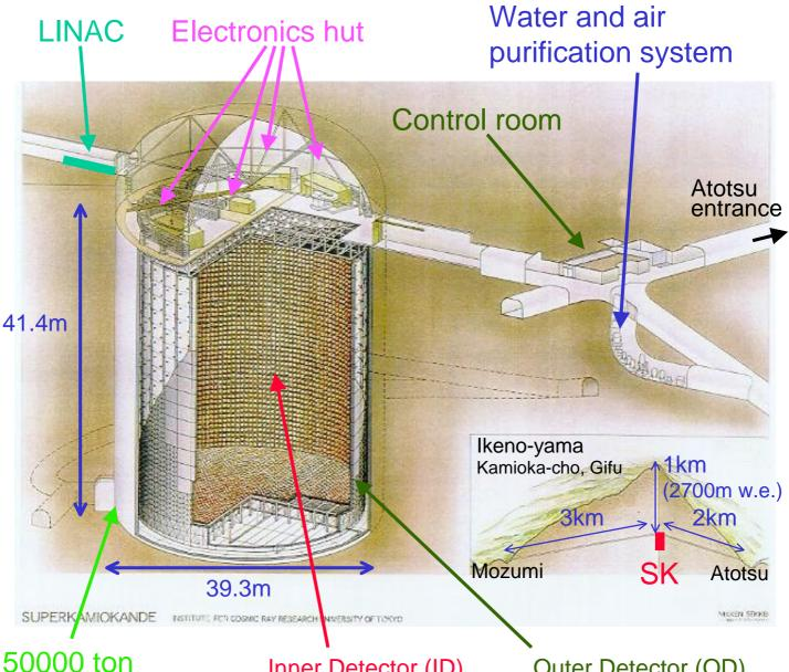
50000 tonInner Detector (ID)Outer Detector (OD)stainless steel tank11146 of 20 inch PMTs1867 of 8 inch PMTs
