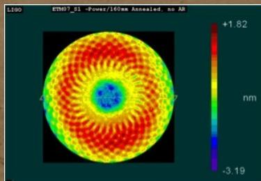
Low absorption fused silica (surface  $< 0.7$  nm RMS, micro-roughness  $< 0.2$  nm RMS, 34 cm diameter 20 cm thickness, 40 kg mass)
