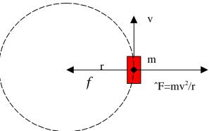
We can determine the banking angle under extreme conditions f = 0 (ice!!), thus not relying on frictional forces.
