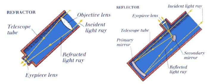
How does the size of a telescope help see more? It can collect more light and give more angular resolution. Telescopes sizes are referred to by the diameter of their primary mirror or lens. (*i.e.* 1 meter, 12 in)
