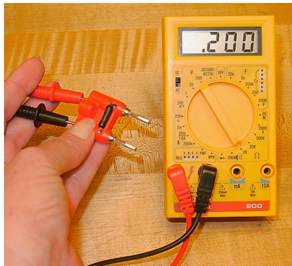
Fig. 10-A: Ohmmeter and Resistor Ohmmeter Reading: 0.200 \text{ k}\Omega = 200 \Omega . Connect ohmmeter to resistor for resistance measurement of an individual element.
