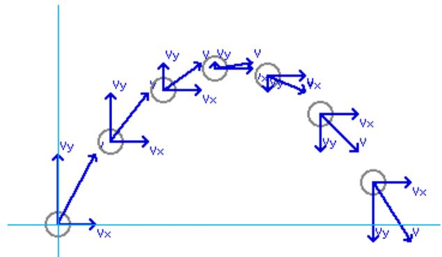
Fig. 4-1 Projectile motion. The trajectory is a parabola.
