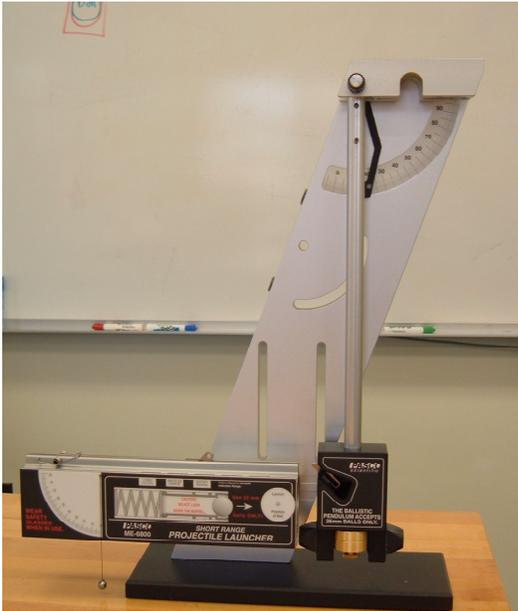
Fig. 8-1 Ballistic Pendulum
